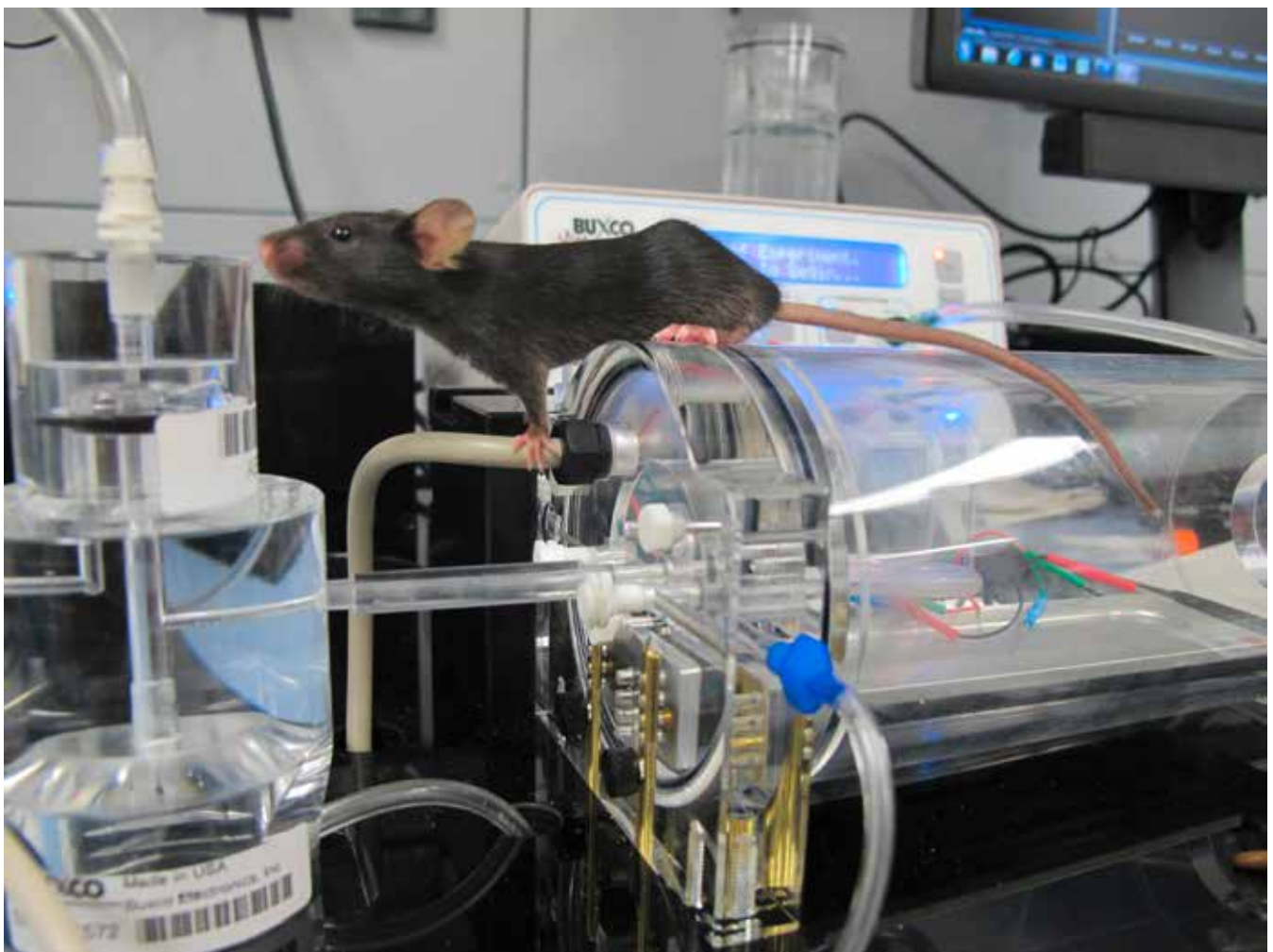
Figure 3. C57BL/6 mouse is interested in the system used for measuring lung function, i.e., determination of airway resistance and its alteration by methacholine (Figure reprinted with kind permission of Dr. M. Wegmann, FZB)
